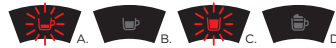
Fig. 34: Luminous alert that there is a lack of water in the water tank.
